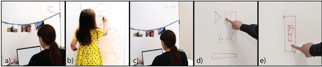
Fig. 11. The panel depicts various technology demonstrations. Panel a) A static notification. Panel b) A static line drawing of the Mona Lisa which users can modify using hand-held light sources. Panel c) A dynamic clock which updates every minute. Panel d) An interactive music menu. Panel e) An interactive light switch.
