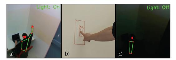
Fig. 8. Panel a) The pose detection of a user touching an element on the photochromic wall. Panel b) The color change of a light switch shape on the photochromic wall. Panel c) The interaction, lights turn off, that occurs from touching the element on the photochromic wall.
