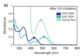
Fig. 3. Absorption data from long-term Yamada DAE-0068, long-term Yamada DAE-0004, and short-term Qingdao's Garnet Red. Panel a) shows the wavelengths at which the different materials activate and panel b) shows the wavelengths at which the long-term Yamada materials deactivate. Data courtesy of Yamada. Optimal activation and deactivation wavelengths are indicated by asterisks.
