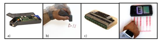
Fig. 12. Panel a) The smart pen 3D printed case, which includes a camera and UV LED. Panel b) The smart pen used to draw and interact with a play button. Panel c) The smartphone case components including LED arrays, mouse sensors, and a time of flight array. Panel d) The smartphone projecting a game controller on a photochromic surface.
