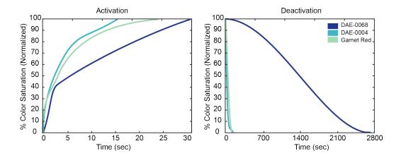
Fig. 4. Activation and deactivation times from the long-term Yamada DAE-0068, long-term Yamada DAE-0004, and short-term Garnet Red. The short-term material lasts for approximately 16 minutes, while the long-term Yamada Red material (DAE-0004) lasts for about 20 minutes, and the long-term Yamada Purple Red (DAE-0068) material lasts for about 6 hours.
